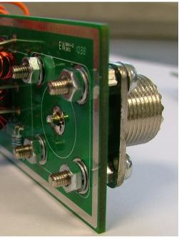
Fit the 8 hex spacers to detector PCB in RF socket fixing positions, note that the thread passes through the PCB and is fixed by a nut and shake-proof washer on the component side of board. Only tighten them "finger" tight at this stage. Temporarily hold the RF connectors in place with 3mm screws and solder the center terminal on the component side of the PCB, straighten the connectors and tighten the 8 fixing nuts.
