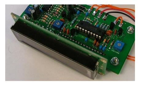
Using 3 short pieces of hook up wire connect the detector PCB with the main board: Connect points RE to REV, GND to GND and FWD to FWD.
