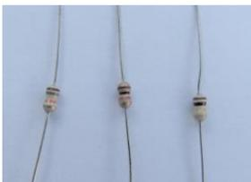
All resistors in this kit have four colour bands, three for value and one for tolerance.
