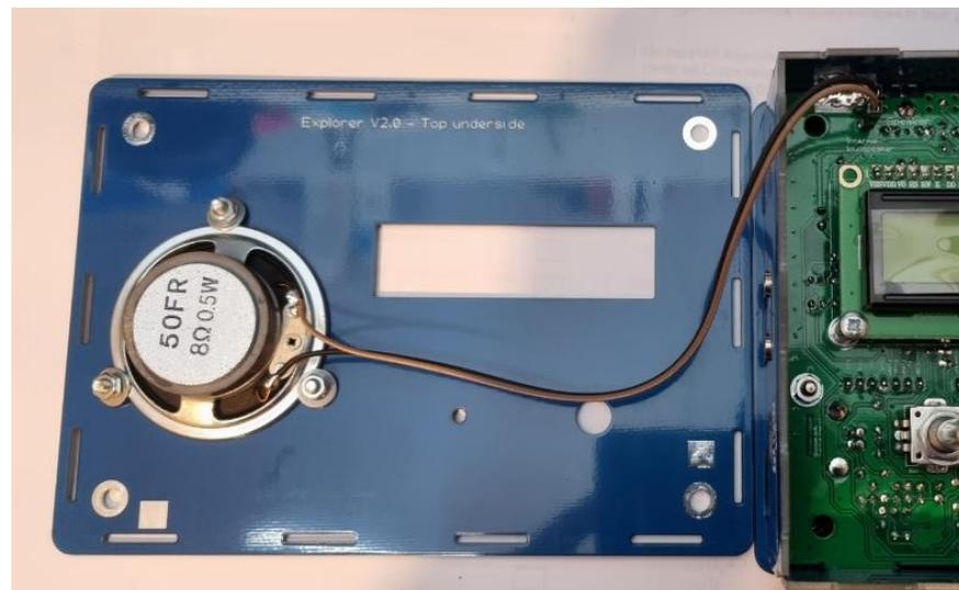
Cut a female socket with about 250mm of wire from each of the pre-terminated jumper leads, solder to each of the two speaker terminals – note polarity and wire colour isn't important.
