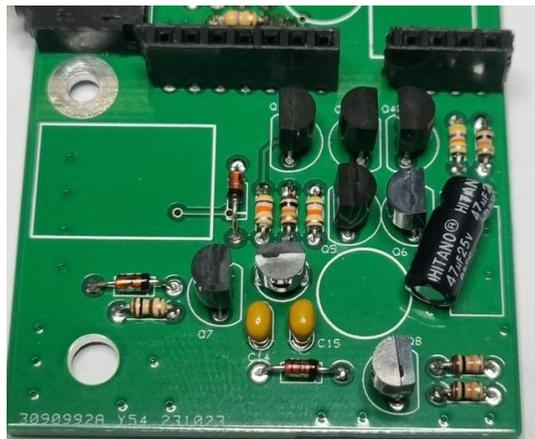
Note C13 is mounted flat to the PCB and at an angle to avoid a clash with components on main PCB.
