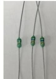
Axial inductors use the same colour code as resistors with their value based in micro Henrys; for example 5.6uH is marked Green (5), Blue (6), Gold (divide by 10) and gold (5% tolerance). All inductors used are larger than resistors so are unlikely to be confused – they won't fit a resistor footprint.
