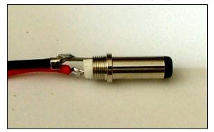
Remove the connector cover and slide over both leads. Solder the positive (+) lead to the center contact and negative (-) to the outer contact and strain relief, when cool, carefully crimp the strain relief over
