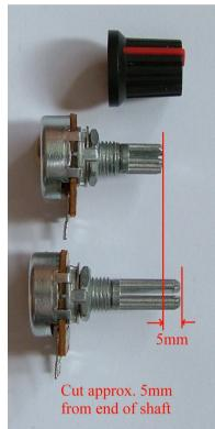
The knobs available for splined potentiometers are designed to be used with thick moulded plastic panels; for the CW adapter to have an attractive finish the potentiometer shafts need modifying. Refer to the photo: hold the unwanted part in a vice (a pair of pliers will suffice if care is used) and cut about 5mm from the shaft using a junior hacksaw, clean off the sharp edges with a small file.
