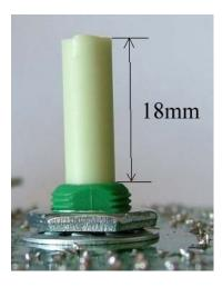
Before fitting VR1 and VR2 cut the shafts to required length, if using the suggested case the shafts need to be cut so that 18mm is left protruding above the mounting thread.
