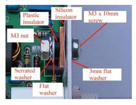
I have catered for two methods of fitting a front panel; with a little thought I'm sure there are many more. For those wanting to design their own front panel critical hole dimensions and spacing are given on the drilling template.
