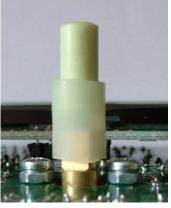
Fit 4 M3 x 12mm hexagonal spacers to the corners of the PCB, a flat and serrated washer should be fitted under each nut
