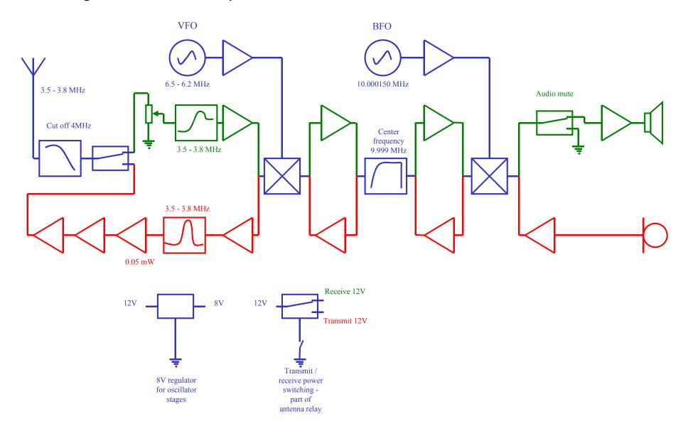
The radio uses a single IF super-heterodyne architecture with several so called bi-directional stages. These allow the sharing of all the main functional blocks between transmit and receive – mixers, IF filter VFO and BFO.
