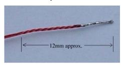
about 30cm long and at one end tightly twist all three together for about 12mm, snip the end off and solder together — this will make it easier to thread the wires
