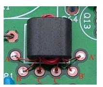
in length and solder in place; be careful to make sure that the enamel burns away and the wire tins properly. Once the first two wires have been soldered in place the other four may be cropped and soldered. After the radio has been completed (and tested) the transformers may be fixed
