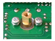
Fit the tuning capacitor using M2.5 x 6mm screws. NOTE: screws must have nuts fitted underneath their heads before fitting so as screw thread doesn't foul the capacitor vanes.
