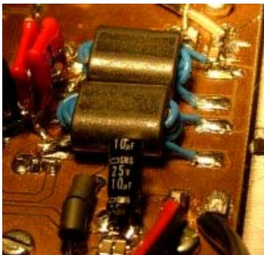
Output transformer mounting detail.
